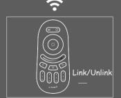
b.Unlink: Long press the(I) button of the linked zone immediately once you switch on the light. The unlink is done once the light blinks 9 times.
