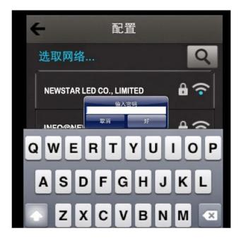
At this time the device will remind to restart the program, please click OK, if the password is correct, so the device connected with the router successfully;
