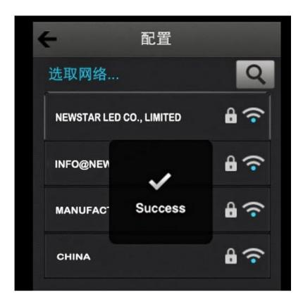
Quit the device list, open Wi-Fi, to connect with the network which WiFi controller is configured successfully,
